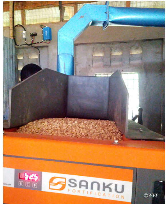
Mixed maize and sorghum passing through a fortifier before milling, Kakuma camp.
